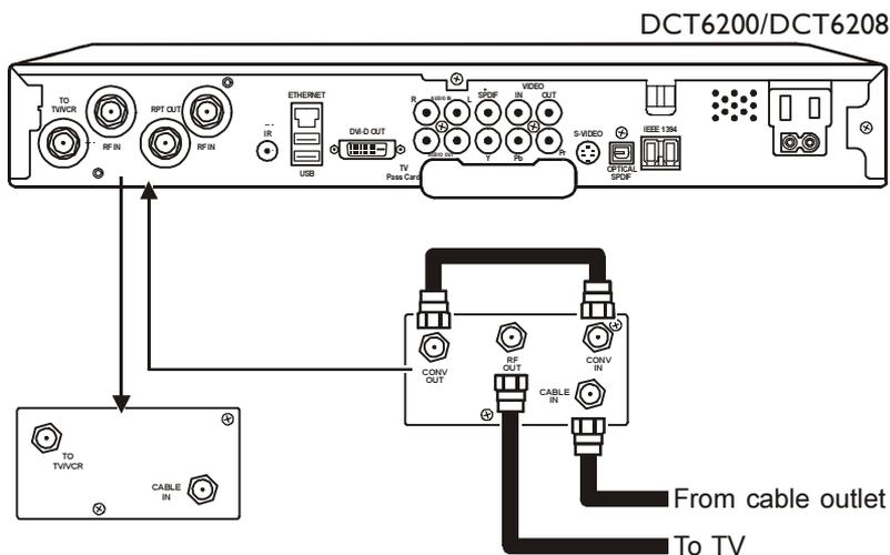
The DCT\* may be equipped with an optional RF Bypass switch.
