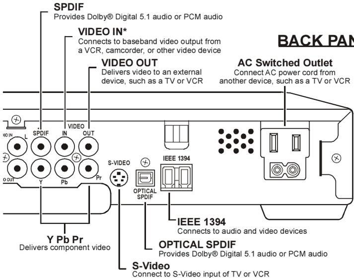
**\*Your DCT6200/DCT6208 may not support all of the inputs and outputs shown.**
